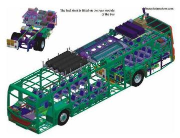
This electricity is used to charge the battery to power the motor of the bus. A number of fuel cells are combined to form a fuel cell stack, which is placed in the rear module of the bus.
